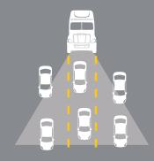
Detroit Assurance Radar reports the distance, velocity, width, lateral offset, type, and confidence level of six vehicles in the truck's path.
