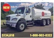
2017 Freightliner M2 106, Cummins ISL 300, 300 HP, Allison 3000 RDS Transmission, 5.29 Ratio, 196" WB, 11R22.5 Tires, New Ledwell 4,000 Gallon Water Tank with Rear Hose Reel, Front, Sid and Rear Discharge. New. (HHJG4317-WFF-2)
