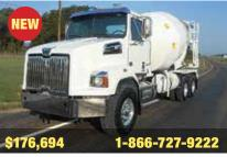
2018 Western Star 4700SB, Rigged w/Becks Industrial 10.5 Cubic Yard Mixer Body, Detroit EW4, Detroit DD13 Engine, 450 HP, Allison 4500 RDS Transmission, 230" WB, 11R22.5 Tires, All Aluminum Wheels, Warranty. New. (JPJN7826--BRY-1)
