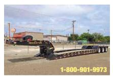
2015 Dynaweld LB55-22D Lowboy, Air Ride Suspension; 53 ft Length x 102 in Width; Apitong Floor; Fixed Tri Axle; Steel Comp New Air Ride 3 Axle Non Ground Bearing RGN with Air Lift 3rd Axle, 55 Ton in 12'. 25' in the Well, 102" Swing Radius. New. (FP105328- SAN-TRL-2)
