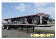
2006 Utility Combo Flatbed, (Qty: 6) Air Ride; 48 ft Length x 102 in Width; LP 24.5 Tires; Fixed Spread Tandem Axle; Combo-Composition; Air Ride, Boxes, with Rear Flip, Aluminum Wheels, Virgin Rubber. (6A815217-TEM-TRL-1)
