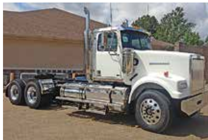
2013 Western Star 4900, Detroit DD15, 505 HP, 10 Spd, Air Ride Suspension, 3.90 Ratio, 220 " Wheelbase, 24.5 Tires, All Aluminum Wheels. New. (DPFA55974-TYL-2)
