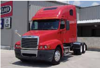
2007 Freightliner CL12064ST Century 120, 70 in Raised Roof Condo; 14.0 Detroit Engine 455 hp; Diesel; 10 Spd OD; Engine Brake; Air Ride; 3.58 Ratio; LP 22.5 Tires; Alum/Steel Wheels; 230 in WB; Tandem Axle, 570,000 Miles. (7LV79710-TEM-2)
