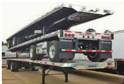
2013 Transcraft Combo Flatbed, (Qty: 3) Air Ride; 48' Long x 102" Wide; Alum. Floor; 22.5 Tires; Alum/Steel Wheels; Spread-tandem Ax; Combo Comp; Sliding winches, Alum. outsiders LED lights. -0-Down WAC. New (D3756676-SHV-TRL-2b)
