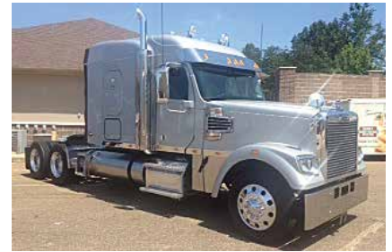
2013 Freightliner Coronado CC132, Detroit DD15, 475 HP, 10 Speed, 3.42 Ratio, Air Ride Suspension, 262" Wheelbase, 24.5 LP Tires, All Aluminum Wheels, Warranty. New. (DDBY8837-TXK-2)
