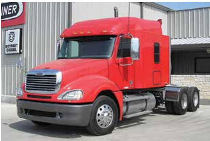
2008 Freightliner CL12064ST Columbia 120 , 70 in Mid Roof XT Sleeper; 14.0 Detroit Engine 515 hp; Diesel; 10 Spd OD; Engine Brake; Air Ride; 3.42 Ratio; LP 22.5 Tires; Aluminum Wheels; 230" WB, 593,000 Miles. (8LZ86155-WAC-2)
