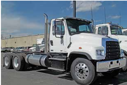
2012 Freightliner 114SD , Detroit DD13, 450 HP, 10 Spd Transmission, TufTrac Suspension, 4.30 Ratio, 220" Wheelbase, Aluminum Front Wheels, Steel Rear Wheels, 24.5 Tires. New. (CHBT4798-FAR-1) $118,200 Includes FET
