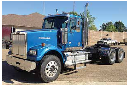
2012 Western Star 4900 , Detroit DD15, 505 HP, 10 Spd, 3.90 Ratio, Engine Brake, 230" Wheelbase Air Ride Suspension, 24.5 Tires, Aluminum Front Wheels, Steel Rear Wheels, Warranty. New. (CPBM9285-TYL-2)
