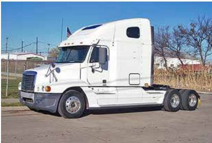
2007 Freightliner CST 12064 Century 120 , 70 in RR Condo; Detroit 455 HP; 10 Spd OD; Engine Brake; Air Ride Suspension; 3.58 Ratio; 22.5LP Tires; All Aluminum Wheels; 236 in Wheelbase; Tandem Axle, 598,000 Miles. (7LX03451-WFF-3)
