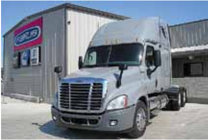
2009 Freightliner CA12564SLP Cascadia, 72 in Raised Roof Condo; 14.0 Detroit 500 hp; Diesel; 10 Spd OD; Engine Brake; Air Ride; 3.42 Ratio; LP 22.5 Tires; Aluminum Wheels; 230 in Wheelbase; Tandem Axle, 379,000 Miles. (9LAA3647-TEM-2)
