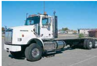
2012 Western Star 4900SA , Det, 475 hp; Diesel; 18 Spd; Eng. Brake; Hendrickson 65000# Solid Susp, 1202A 2-spd Aux. trans.; 5.38 R; 24.5 Tires; Alum/Stl Whls; 320" WB; 22,000 lb Frnt Ax Wt; 58,000 lb Rear Ax Wt. New. (CPBM9897-FAR-3)
