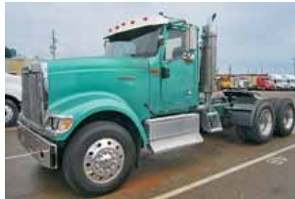
2000 International 9900, Caterpillar C12, 430 HP, 10 Spd Transmission Air Ride Suspension, 24.5 Tires, Aluminum Front Wheels, Aluminum Outer Rear Wheels. (YCO66784-TYL-2) $23,500
