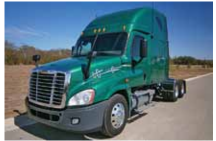
2009 Freightliner CA12564SLP Cascadia , 72 in Raised Roof Condo; 14.0 Detroit Engine 500 hp; Diesel; 10 Spd OD; Engine Brake; Air Ride Suspension; 3.42 Ratio; LP 22.5 Tires; All Aluminum Wheels; 230 in Wheelbase; Tandem Axle, Thermo King APU, 357,000 Miles. (9LAF0076-BRY-3)
