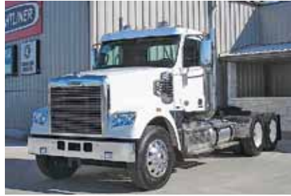
2012 Freightliner CC12264 Coronado, DD 15 Detroit Engine 475 hp; Diesel; 10 Spd OD; Engine Brake; Air Ride Suspension; 3.58 Ratio; 11 R 24.5 Tires; Aluminum/Steel Wheels; 220 in Wheelbase; Tandem Axle. New (CDBM5400-TEM-3)
