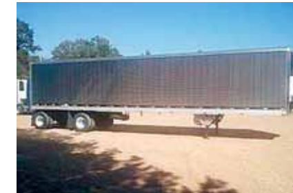
2008 Utility Reefer, Air Ride Suspension; 48 ft Length x 102 in Width; Aluminum Floor; 22.5 Tires; Aluminum Wheels; Spread Tandem Axle; Utility Reefer. 48x102 Stainless package. Spread Air Ride. (8U538101-SHV-TRL-3c)
