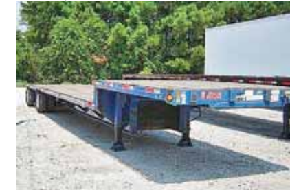
2000 Fontaine Drop Deck, (Qty: 6) Air Ride; 48 ft Long / 102 in Dide; Apitong Floor; 22.5 Tires; Steel Disc Wheels; Spread Tandem Ax; Steel Comp.; Wide Spread Air ride, Container locks 1-20' container. Trailer has 11' upper deck / 37' bottom deck. (Y5993414-SHV-TRL-1A) Call for Price
