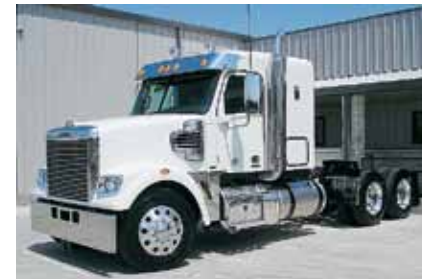
2012 Freightliner CC11264 Coronado SD, 48 in Mid Roof Sleeper; DD 15 Detroit Engine 505 hp; Diesel; 10 Spd OD; Engine Brake; Air Ride; 3.42 Ratio; 11R 24.5 Tires; Aluminum Wheels; 230 in Wheelbase; Tandem Axle. (BH5652-WAC-2)
