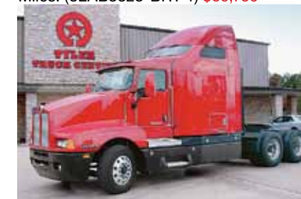
2007 Kenworth T600, 72 in Aerocab Aerodyne Sleeper; ISX Cummins Engine 450 hp; Diesel; Automatic OD; Engine Brake; Air Ride; 3.36 Ratio; 22.5 LP Tires; All Aluminum Wheels; 240 in Wheelbase. (7J189869-SHV-1) $49,700 $48,500
